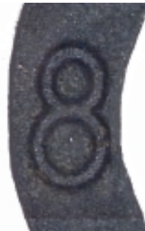
PPS Bushing Prototype, 8-cavity Production Mold
